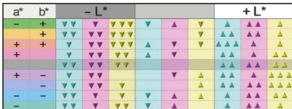
FIGURE E11: Chart showing how to move C, M and Y inks in response to +/- Lab errors.
